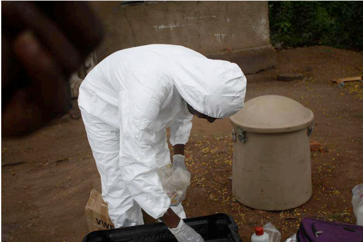
The PREDICT Tanzania team packs up equipment after collecting specimens from rodents. The mushroom shaped container in the background is a specially designed transport container for LN2 dryshippers, ensuring the Dryshipper container is well protected during overland or air travel, and that all stored specimens are well within the temperature range required for viral isolation. Photo by Liz Vanwormer.
